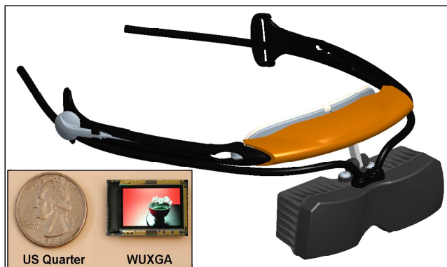
Figure 1. Binocular 3D stereoscopic HMD using full color WUXGA resolution AMOLED microdisplay (inset).
