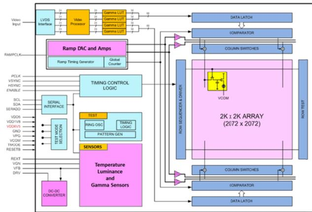
Figure 2. 2K x 2K block diagram.
