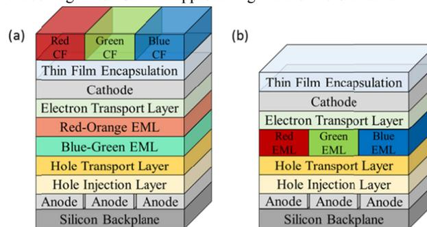
**Figure 1.** Structure of (a) conventional white OLED with color filter (CF) array in comparison with a (b) directly patterned OLED with red, green and blue emitter layers (EML) eliminating the need for color filters. From Ref 8.
