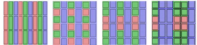
Figure 4. Examples of 3 x 3 color pixel configurations.
