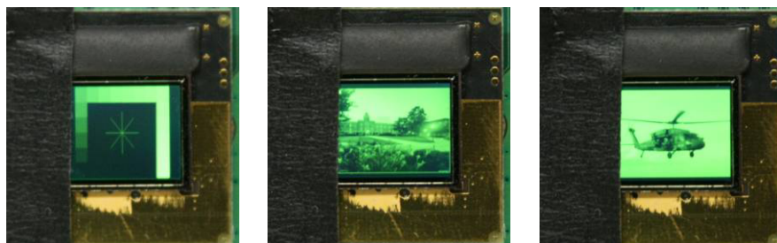
Figure 6. The High Brightness Green SXGA-2 display showing the Grayscale pattern and two pictures. Black masking tape was placed over the bright calibration bar on the left side of the screen for all tests.
