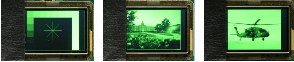
Figure 15. The High Brightness Green WUXGA display showing the Grayscale pattern and two pictures. Black masking tape was placed over the bright calibration bar on the left side of the screen for uniformity and qualitative tests. Black flocking material was placed over calibration bar for contrast measurements.
